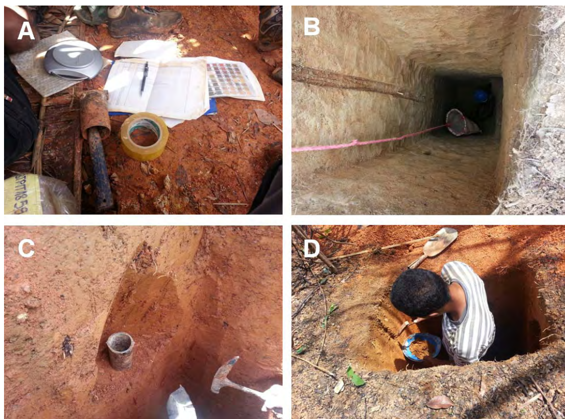
Figure 9-3: Photos of work undertaken in the field. A. Geologists field tools and protocols; B. Ongoing pit showing the typical sampling trench and branches inserted to track the depth within pits. C. Ledge cut into the side of the pit used to collect the sample for density measurements. D. Geologist sampling the first meter within a pit.
