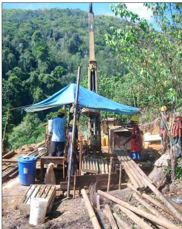
Figure 10-1: Photograph of the Versadrill Kmb.4km drill rig in operation (Gilbertson, 2013)
