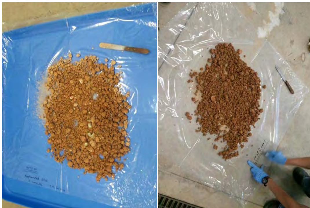
Figure 13-4: Column Tests Agglomerated Feed - Column 1 (left) and Column 2 (right)
