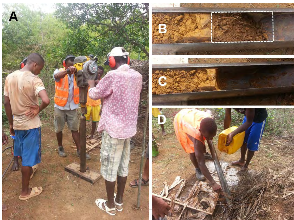
Figure 9-5: Window sampler demonstration. A. Window sampler in action. B. Sample tube with fall back material from previous meter (in white box). C. Contaminated material removed. D. Cleaning of sample tube prior to next run.
